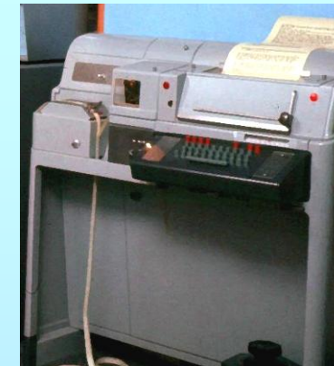
Model 28ASR from Teletype, the Cadillac of RTTY machines in the 1960s.
